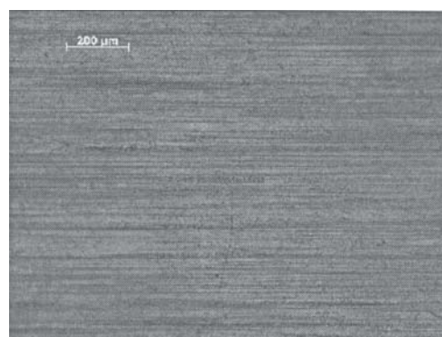
The photo corresponding for nickel electrodeposition process with sodium saccharine and sodium lauryl sulfate in Watts' bath
